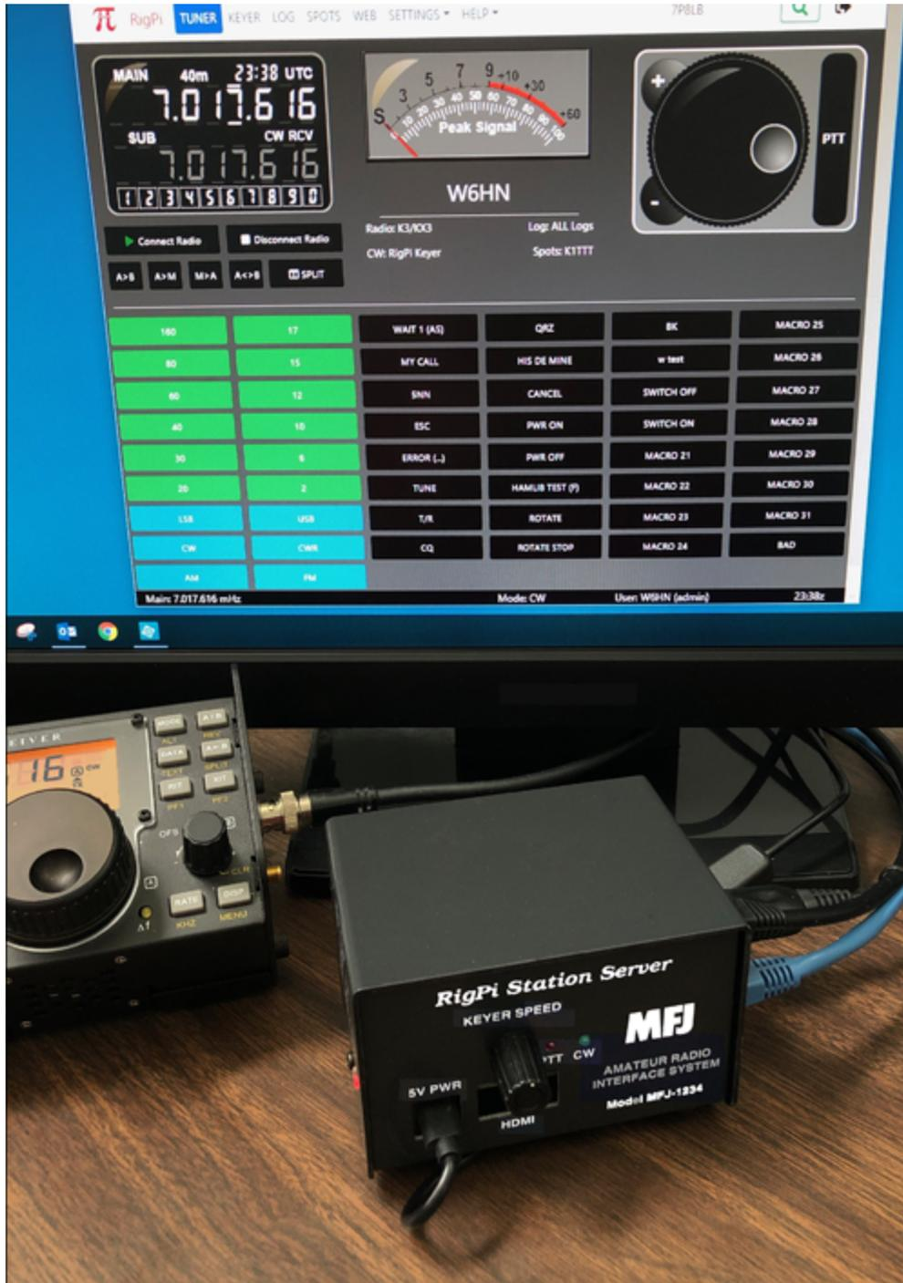
RigPi Station Server (RSS) is a computer system designed to control your station and facilitate on-the-air activities. RSS introduces a radically new way of station control by using a server model for allowing multiple users and radios to be accommodated simultaneously through standard Internet browsers.
