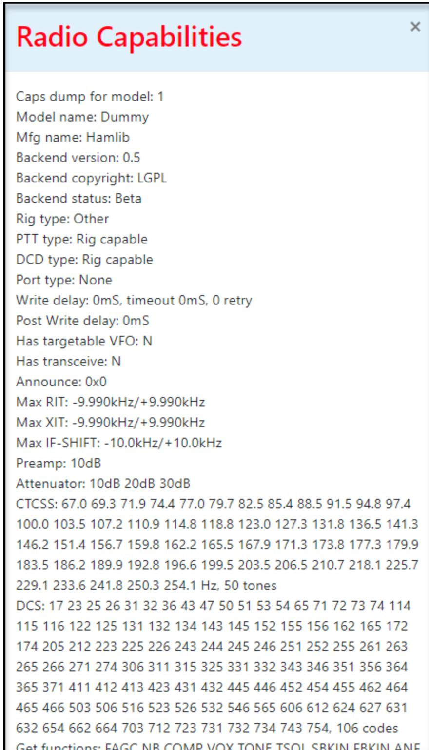
Go to RigPi SETTINGS>Radio>Advanced and use the Radio Capabilities button to show a list of all features for the selected radio supported by Hamlib.
