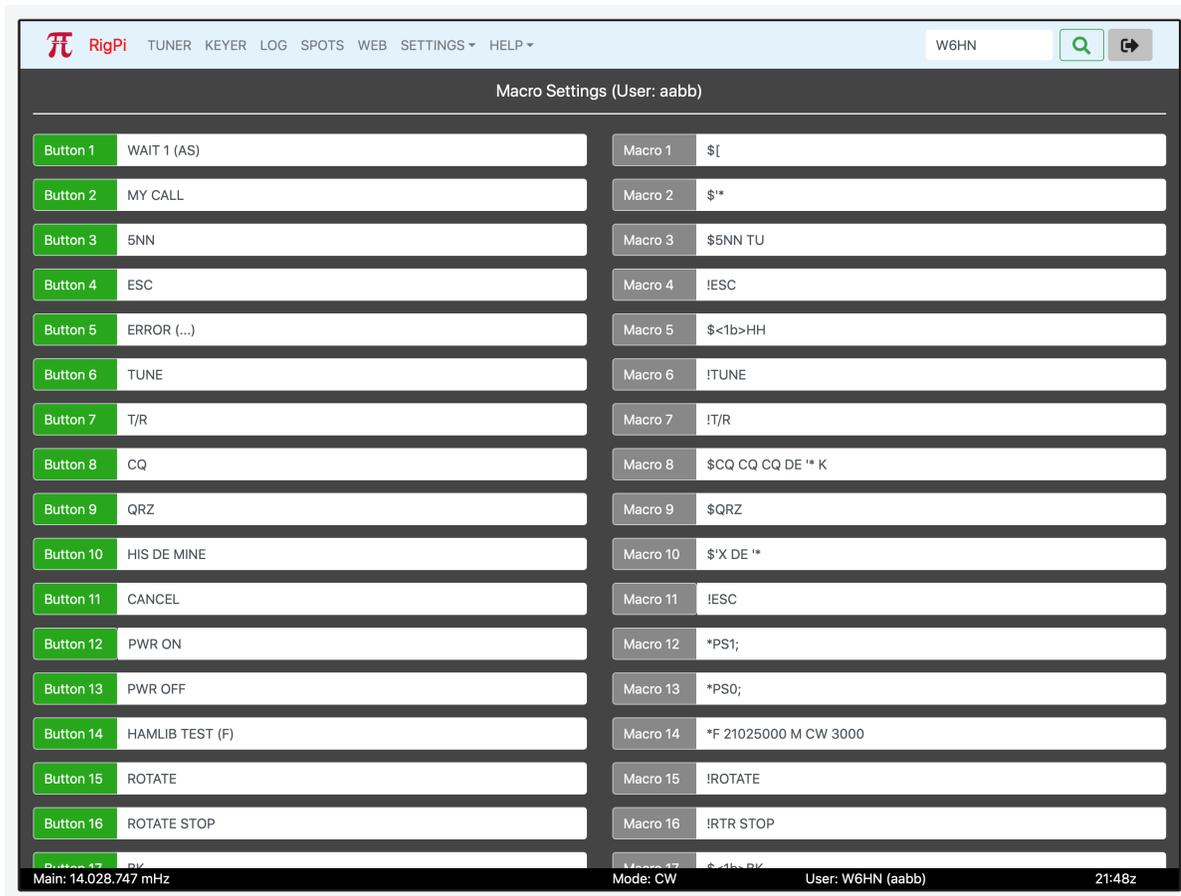
RSS provides 32 programmable macro keys. The keys are available in the Tuner and CW Keyer windows. Each macro has a space to enter a button caption and a command. The total length of all macros is 2000 characters per account. Macros can be used in a number of ways:
