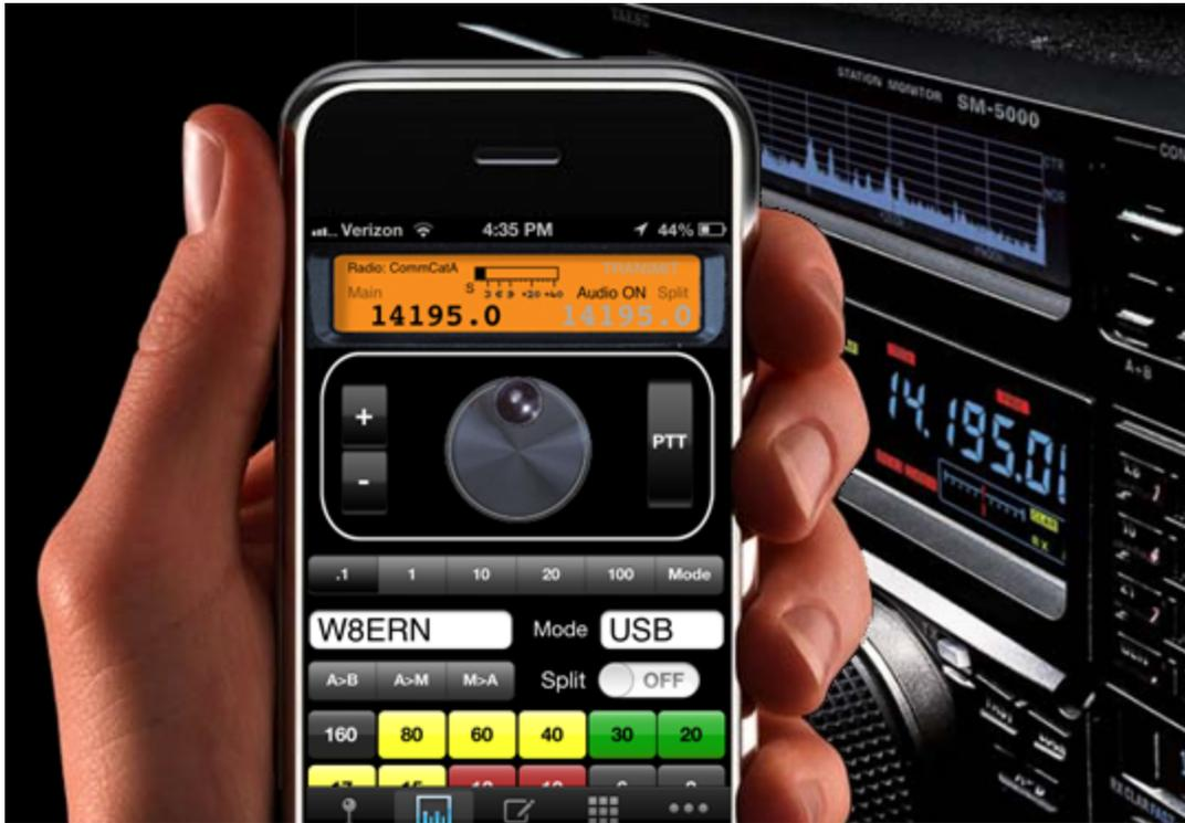
In addition to browser access, CommCat Mobile for iOS and [CommCat](#) for Windows can connect to RSS for radio control.
