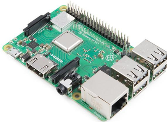
RSS is based on a Raspberry Pi computer running Linux plus RigPi Keyer and RigPi Audio boards. RigPi Keyer uses the popular K1EL WinKeyer chip for keyboard or paddle input. RigPi Audio is used for Voice-Over IP (VoIP) and remote operations, or for digital modes and I/Q spectral display (panadapter).
